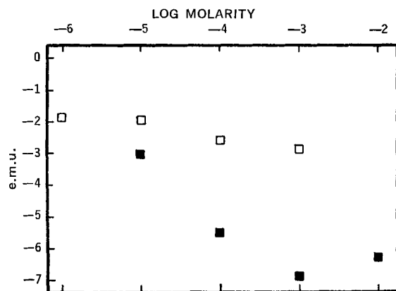
Figure 6—Concentration-mobility profile of cholesterol-sodium taurocholate systems at pH 6.8 showing the effect of purity of commercial samples: Sample A (□) and Sample B (■).
